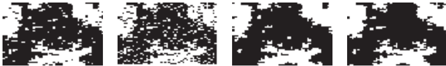
Fig. 17. From the left to the right , the 50 \times 50 original image generated at T_s = 2.15 , degraded images ( p_\tau = 0.1 ), and the restored image by the thermal MPM estimation, and the restored image by the quantum MPM estimation. Each bit-error rate is p_b = 0.06120 for the thermal MPM at T_m = T_s = 2.15 and p_b = 0.06040 for the quantum MPM estimation with \Gamma = 0.8 (at the nearest point from the solution of m_0 = m(\Gamma) ), respectively
